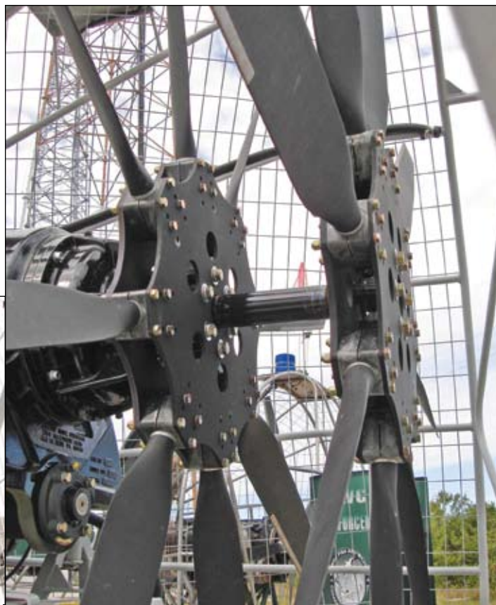
The stainless steel mufflers on the 454 big block Chevy engine, and the counter rotating props with a CH-3 2.3:1 gear reduction are what make this run quieter than most other airboats.
